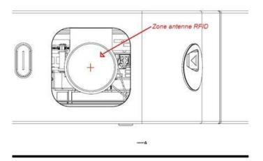
The Reference of the PCD Zero point is the center of the antenna coil
